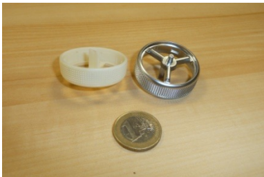
WZ "Chromring", 4-fold Customer: KTB Material: ABS Shape structure: 446 x 396 x 320 mm Direct injection with open nozzles 8 sliders per FN for outer contour
