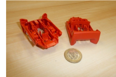
WZ "pressure button", 8-fold Customer: TRW (ZF) Material: POM Shape structure: 512 x 546 x 490 mm Direct injection with open nozzles 8 mech. pusher 8 replaceable shield sliders 8 interchangeable inclined sliders
