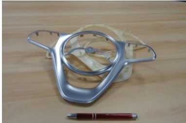
WZ "Aperture Luxury", 1-fold Customer: KTB Material: ABS Shape structure: 496 x 596 x 606 mm 7 Slanted slider
