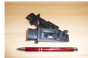
WZ "HFM7 enclosure", 4-fold Customer: Hardener Material: PBT GF30 Shape structure: 446 x 546 x 572 mm Direct injection 4x hydr. NV nozzles 1 hydraulically operated slider per FN DS Hydraulically operated slide lock AS
