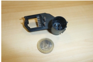
Round table WZ "Connector ASM", 4-fold Customer: Doduco Material: PET Shape structure: 366 x 396 x 450 mm Injection via 4 open HD nozzles Pneumatically operated holder DS
