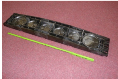
WZ "shaft frame element", 2-fold Customer: Langmatz Material: PC GF 6% (TSG foam) Item weight: 8.5 kg per part Shape structure: 1420 x 746 x 910 mm Direct injection with 6 hydr. NV nozzles Weight Shape: 4.7t
