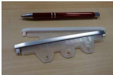
2K-WZ "Divinder Bar" 4+4-fold (4 pcs falling) Customer: KTB Material: ABS+PC / PC Shape structure: 496 x 596 x 465 mm 3 underfloor sliders per FN AS
