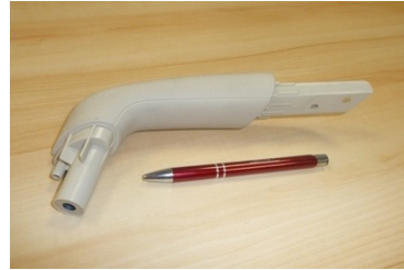
2K-WZ "TZZG-Grundkörper" 2+2-fold (1+1 fold falling) Customer: Utescheny Material: ABS+PC / TPU Shape structure: 596 x 896 x 640 mm Gas internal pressure technology
