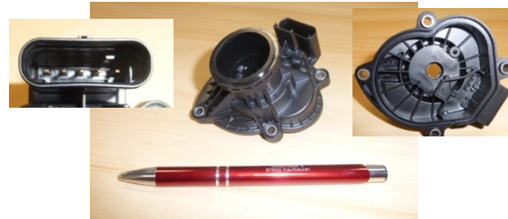
Round table WZ "AGR motor housing", 2+2-fold Customer: Swoboda Material: PPS GF40 Shape structure: 496 x 696 x 615 mm 2FN VU + 2FN HU (each AS) with integrated VU Punching process in the WZ
