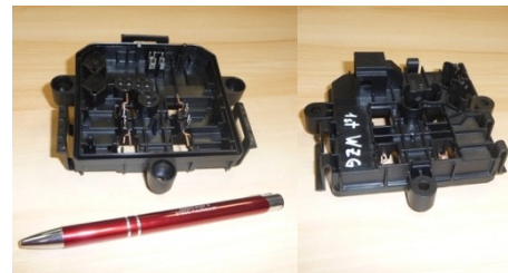
WZ "Airmax Enclosure", 2-fold Customer: Hardener Material: PA66 GF30 Shape structure: 446 x 546 x 547 mm 2 hydraulically operated NV nozzles 1 hydraulically operated slider
